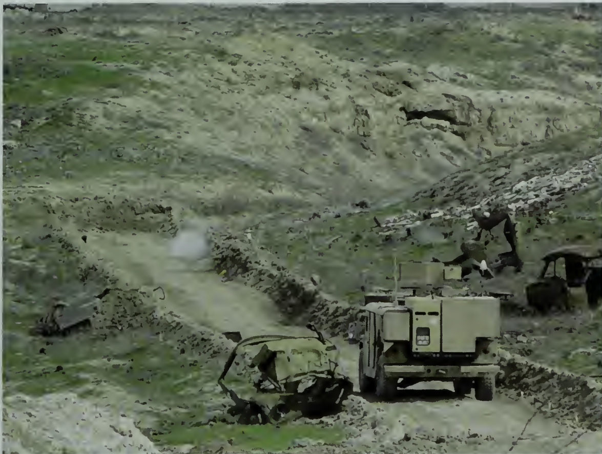
Fig. 6-10. Introduced to the public in December 2002, the ZEUS laser neutralization system is a laser system designed to heat a target until the ordnance explodes. The prototype ZEUS deployed to Afghanistan in March 2003 to neutralize land mines and unexploded ordnance
